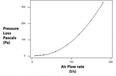
\*Pressure losses with Control Disk 10mm open
