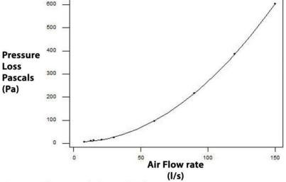
\*Pressure losses with Control Disk 10mm open
