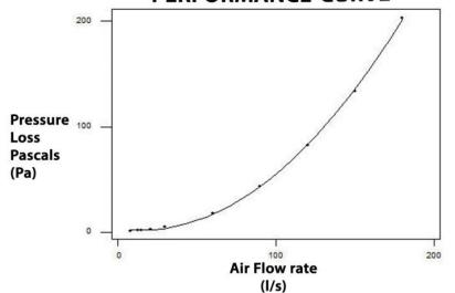
\*Pressure losses with Control Disk 10mm open
