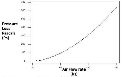
\*Pressure losses with Control Disk 10mm open
