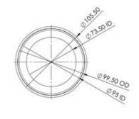
MANUFACTURER: **VERPLAS LTD** PART NUMBER: EK0082 100mm SIZE: FOR USE WITH: VERPLAS SYSTEM 100 **BOX QUANTITY:** 180 INDIVIDUAL WEIGHT: 50g COLOUR White MIN OPERATING TEMP -15°C +60°C MAX OPERATING TEMP
