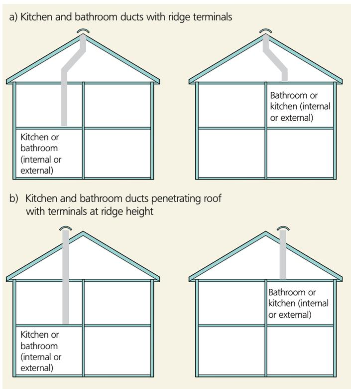
Figure 7 Suitable layouts for passive stack systems
