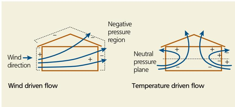
**Figure 2** Schematic showing wind and temperature driven ventilation
