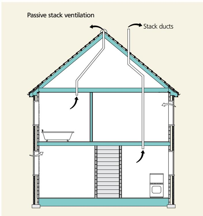
Figure 6 Passive stack ventilation
