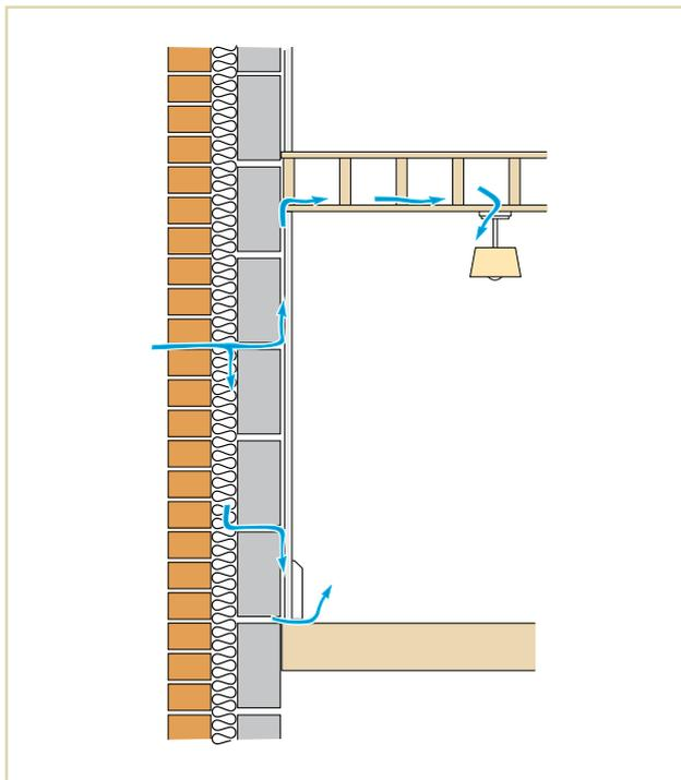
Figure 5 Indirect air leakage paths
