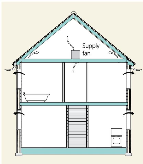
Figure 11 Positive input ventilation (PIV)
