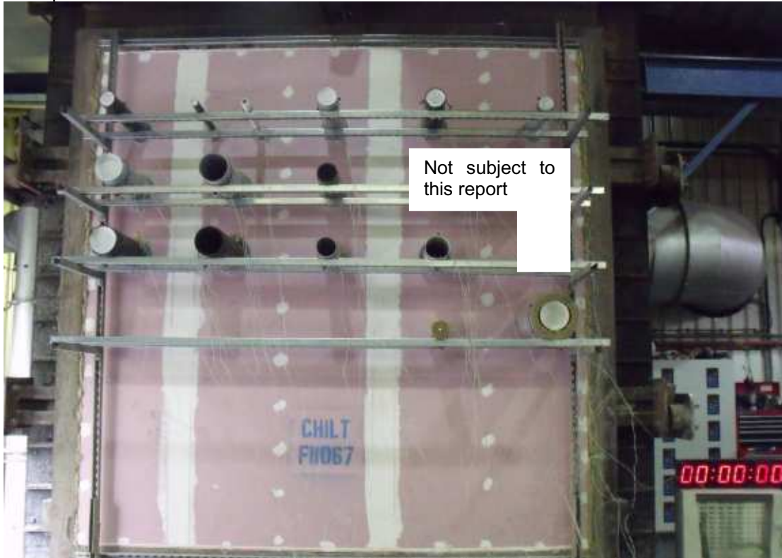
Unexposed face at start of test
